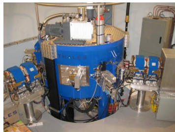
THALES Cyclotron with D-Pace Designed Custom Compact Beamlines, Radiation Shielding, Target Helium Cooling System**, and Load/Unload Process Cabinet with Overpressure**.
